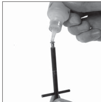
Position a nipple on the spoke wrench and stick it using thread lock M40315. Insert the nipple and wrench into the rim hole and screw the nipple 2 turns onto the previously inserted spoke.
