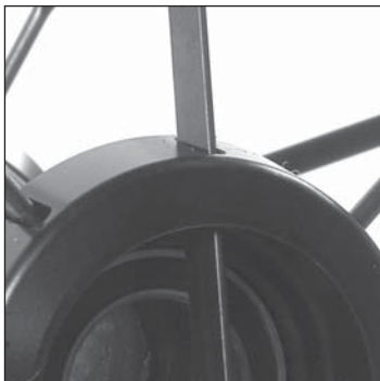
Place a 270 mm spoke (323 902 01) into a hub hole on the non drive side.
